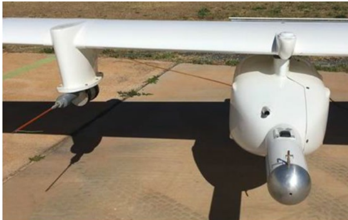
MetPod with the 3D-turbulence probe and internally mounted LiCOR LI-7500 (CO 2 ) and MetOne particle counter mounted on one of the wing pylons
