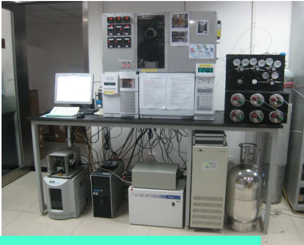
Medusa-GC/MS, technique developed by AGAGE
