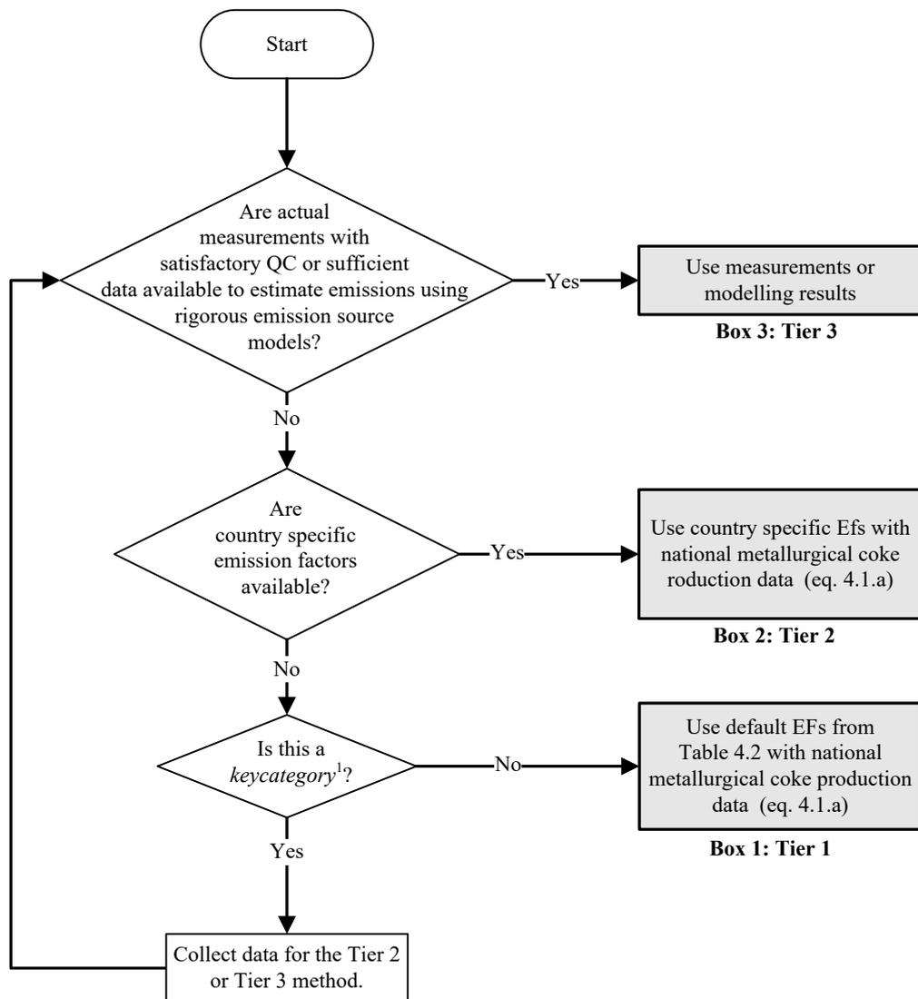
**Figure 4.8b (Updated) Decision tree for estimation of CH<sub>4</sub> emissions from iron and steel production**
