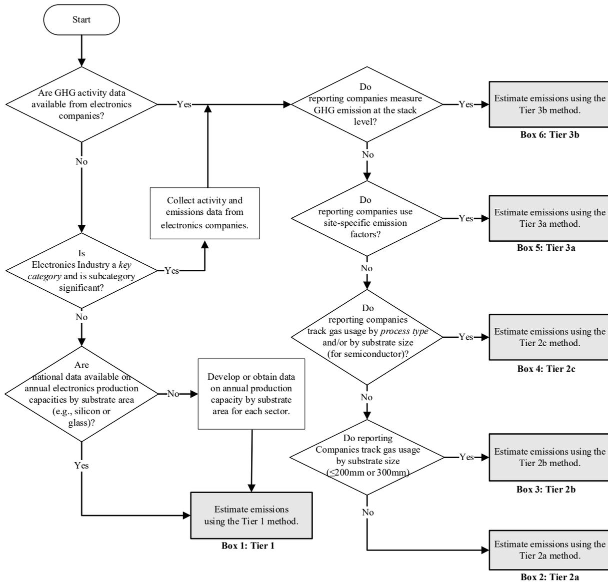
For semiconductor 450 mm substrate size, facilities should test and develop measured emission factors (Tier 3a). Tier 2a should not be used for 450 mm. Measured factors can be phased in over time; previous generation Tier 2c default factors can be used during the phase in period. Tier 3a measured factors should be submitted to IPCC EFDB to allow development of Tier 2 defaults. See section “Adapting Tier 2 Methods to account for technological changes” for more details.
