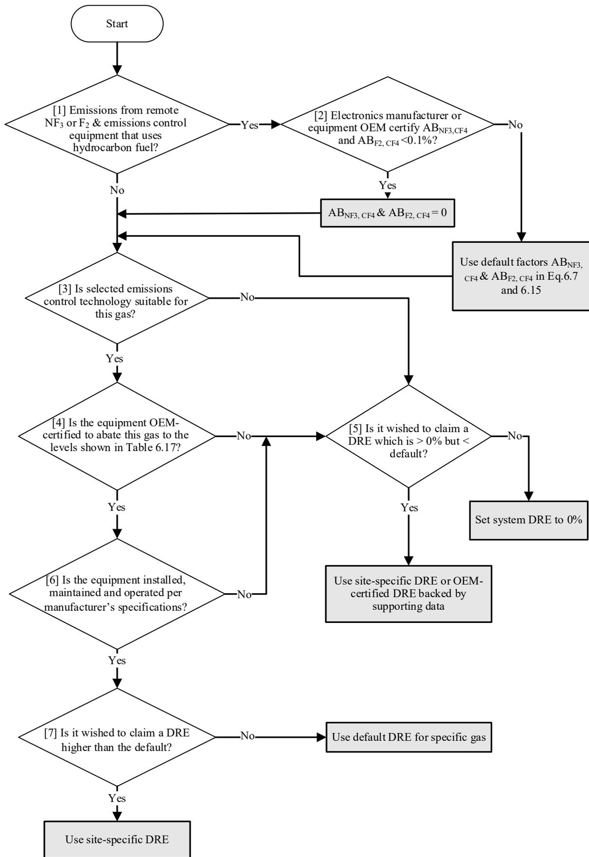
Note: references to equipment in the above figure mean emission control equipment.
