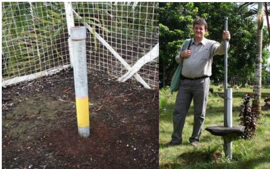
Fig. e. Left: Example of subsidence pole installed in late 2007, 10 years after initial drainage, in PT TH Indo Plantations, Riau, Indonesia and Right: A subsidence pole inserted in deep peat at Woodman Plantations. At the time of this photograph (2011), the pole was installed 8 years prior to the photograph and about 50 cm of subsidence had occurred (Image: Marcel Silvius).
