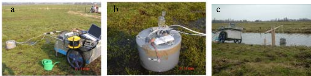
Fig 2. Example of a portable enclosure, connected to a gas analyser and a computer (a). The enclosure is equipped with a water lock to avoid pressure differences and a filter for water vapour to avoid cross-interferences (b). The system can be used to measure CO 2 , CH 4 and N 2 O on land or on water (a and c) (Images A. Schrier-Uijl)
