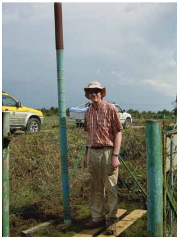
Figure 10: Subsidence pole inserted in peatland in Johor, peninsular Malaysia. The pole was inserted beside an oil palm plantation in 1978 and at the time of this photograph (2007), 2.3 m of subsidence had occurred (the human “measuring stick,” Dr. Chris Banks, is 2 m tall). (Image: J. Jauhiainen).
