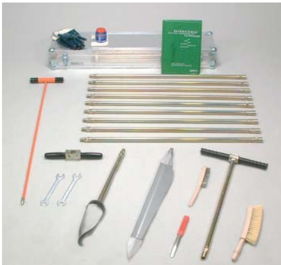
Fig. e. Peat sampler set. Source; www.eijkelkamp.com
