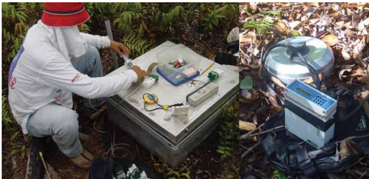
Figure 7: Closed chamber measurements being made in the field; large static chamber (left) and dynamic chamber and CO 2 analyzer (right; images: J. Jauhiainen).
