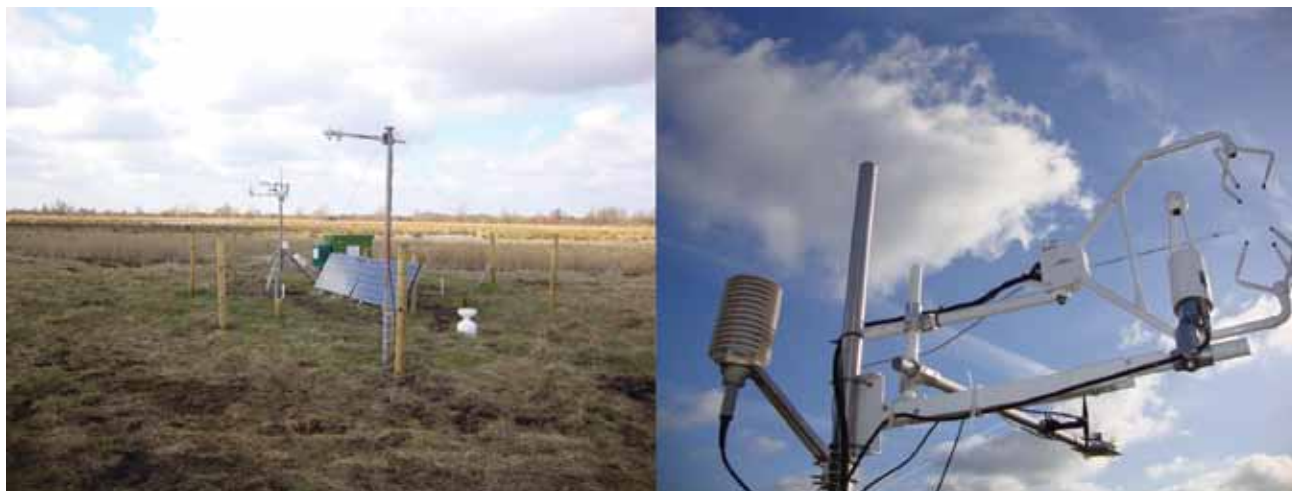
Figure 8: An eddy covariance flux tower measuring surface-atmosphere exchanges of \text{CO}_2 , water and energy at a restored fen peatland in the United Kingdom (left). Eddy covariance instrumentation, consisting of a sonic anemometer, an infrared gas analyzer, and sensors for measuring photosynthetically active radiation, air temperature and relative humidity (right). (Images: R. Morrison).
