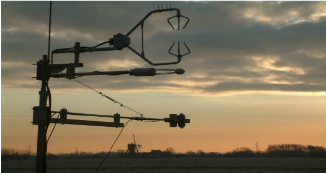
Fig. 5. An eddy covariance system, equipped with sensors for irradiation, wind, temperature, CO 2 and water vapour (Image E. Veenendaal).
