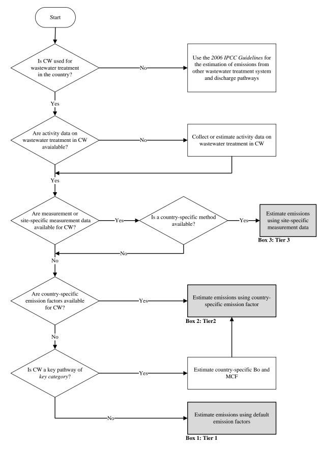
Figure 6.3 Decision tree for CH<sub>4</sub> emissions from constructed wetlands
